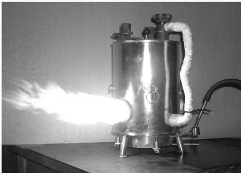
Fig. 1. Burner-demonstrator of power 20 kW.
